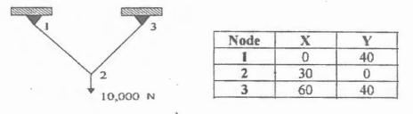
A. Find the joint displacements at 2. Find the stress in the elements.
